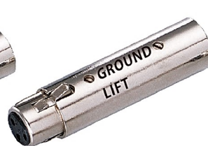
SVP559-GOPEN Female XLR to Male XLR Pin 1 Open for Ground-Loop Can Cancel "Ham Noise" ※ Cable need follow AES48 standard.
