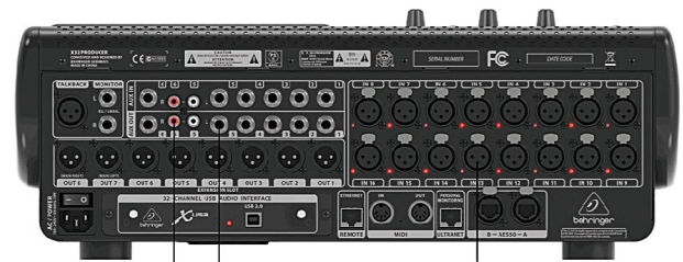
RCA Socket For AV/Tape In TS Socket For Professional Mixer XLR Socket For Professional Mixer
